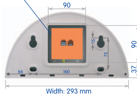
Space for RJ45 wall outlet
