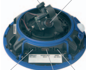
Ethernet In/Out / RS232 ISDN
